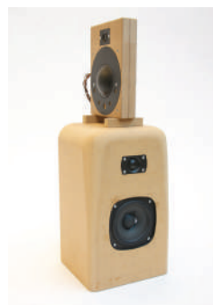
Fig. 4 The "Sharkfin" experimental loudspeaker with a top-mounted dipole made with back-to-back drivers.
