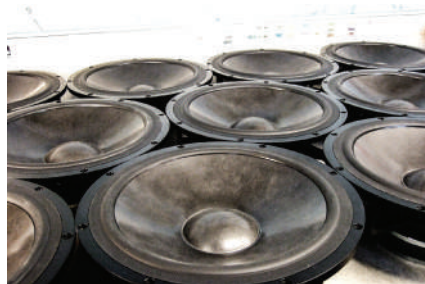
15" drivers, with Rockport Technologies own Carbon Fiber Cone.
