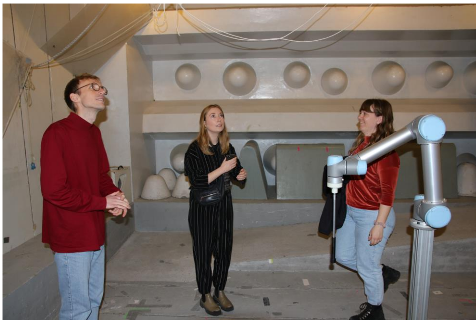
Figure 1: Use of robotics (Universal Robots) in measurements in Reverberation Room, DTU
